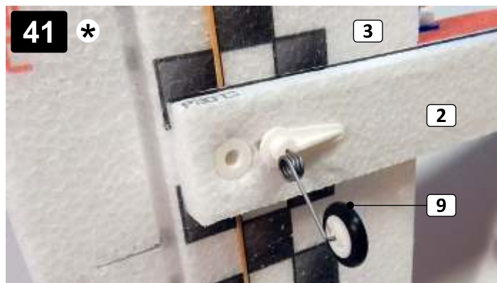
41 * Ostruhu (9) zatlačte zcela do trupu (2) ... Slip in the tailwheel (9) to the fuselage (2) fully ...
